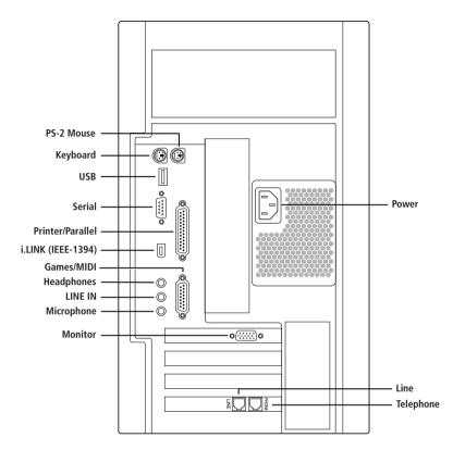
For your convenience, your computer includes USB and i.LINK connectors on both the front and back panels, allowing you to connect to either set of connectors. The i.LINK connector on the back of your system is a 6-pin connector.
